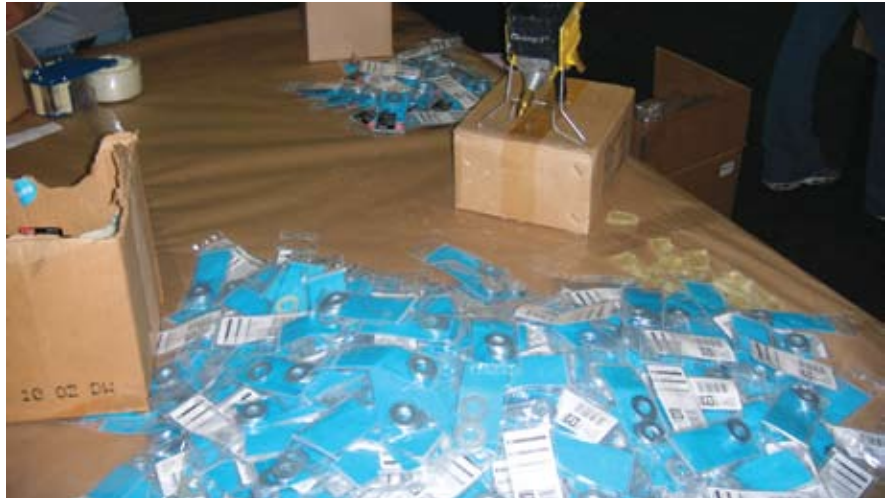
▲ STICKERS ISSUE. A shipment of washer packages arrives at Premier Packaging with the product information stickers becoming dislodged from the bags. The stickers are reattached to the bags using hot-melt glue, and the packages are shipped to Walmart stores.
