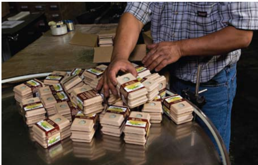
▲ SOAP BUNDLES. In an example of the highly customized hand-assembly work done at Premier Packaging, soap bars are packed into windowed cartons, bound with a branded band, and prepared for distribution to retail stores. The new cartons are made of recycled materials and baby's breath.
